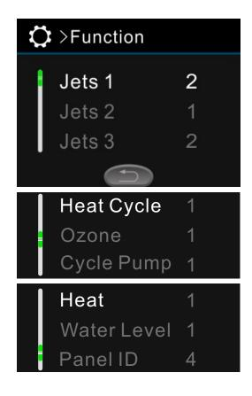
To panel ID, it can be set as 1, 2, 3, or 4. These numbers are used to differ different control panels and the control panel ID must be unique. To other loads, if the figure in "  $\square$ " is 1, then this load has been set. If the figure in "  $\square$ " is 0, then the load is invalid.
