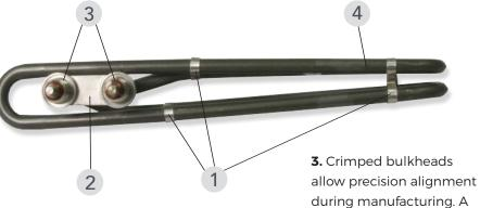
chemically-inert epoxy seal, instead of brazing, improves corrosion resistance. Each assembly is tested to 60 psi, assuring a leak-free installation.
