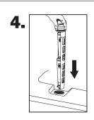
Slowly insert holder into system (see diagrams). Line up holder arrow-(1) with system arrow-(2). Push down until holder tabs-(3) go past system tabs-(4) and turn holder to the right (clockwise) until it stops. To ensure a locked position, attempt to pull holder up. If it stays in place, the lock is secure.
