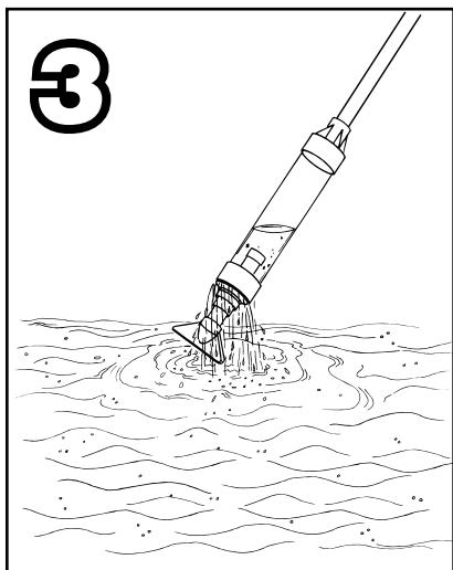
...lift out of the water. Clean filtered water automatically drains out and debris stays in the chamber!
